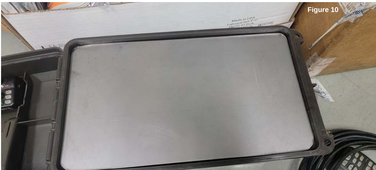
Figure 10: Flat plate fitted on carrying case, before mounting radio, feet and additional finishing
