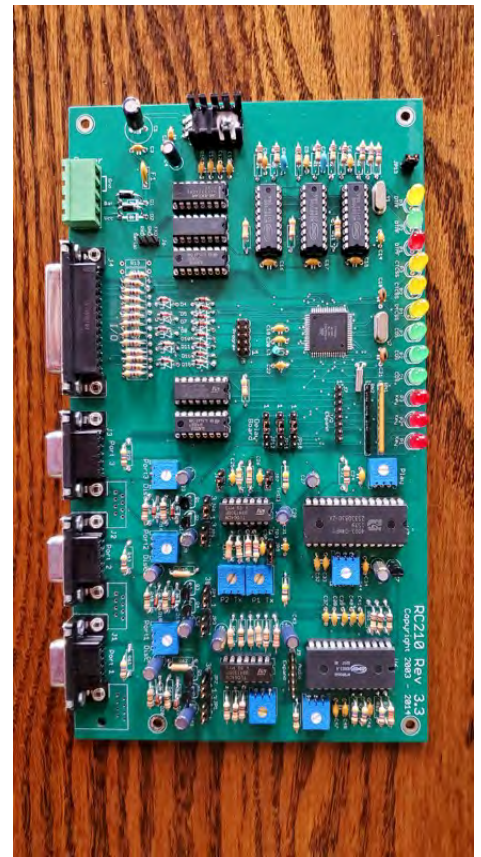
above... One of the completed controller boards for the KARS new repeaters.
