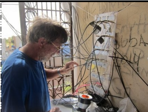
John W2GD on location at Navassa Island K1N selects an antenna at the lexan RF patch panels built by KARS members N9IO and KC9QPM right here in Kankakee County. These are the same panels used one year ago on the FT5ZM Amsterdam Island DXpedition!
