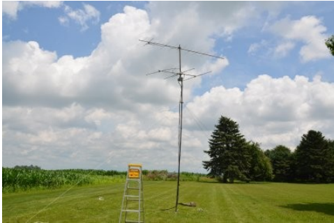
Sections of fiberglass poles supporting the 6 and 2 meter Yagi's
