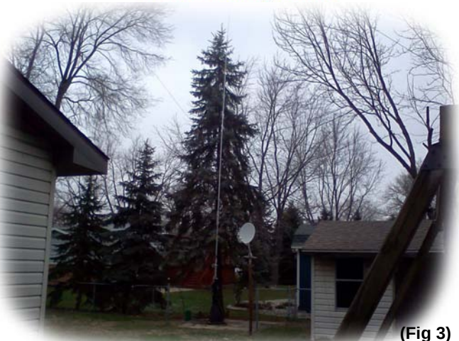
Hinge mounted HF2V 40/80m (above ground) Vertical (Fig 3)
