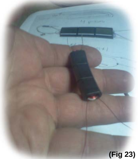
Transformer (pri / sec) winding completed
