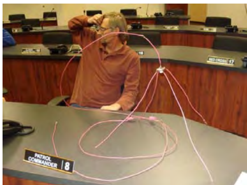
John N9LYE brought a simple 2 meter wire collinear antenna for use at home and in the field
