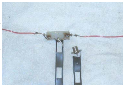
N9LYE's version of the popular G5RV antenna...illustrating the feed point
