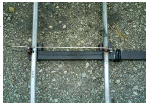
Close-up view of the stub-style feed system
