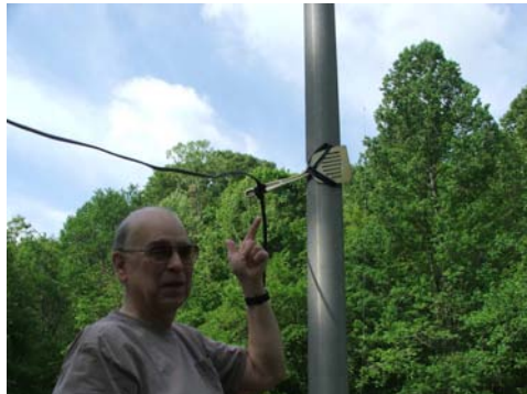
Howard AK9F, demonstrates that necessity is indeed the mother of invention as he points to the "spatula" standoff insulator
