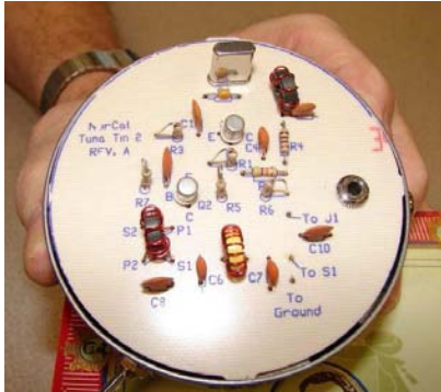
A closeup shot of Duane KB9ZQU's "Tuna Tin Special" QRP transmitter. You can still homebrew a rig to work the world! Nice work Duane!
