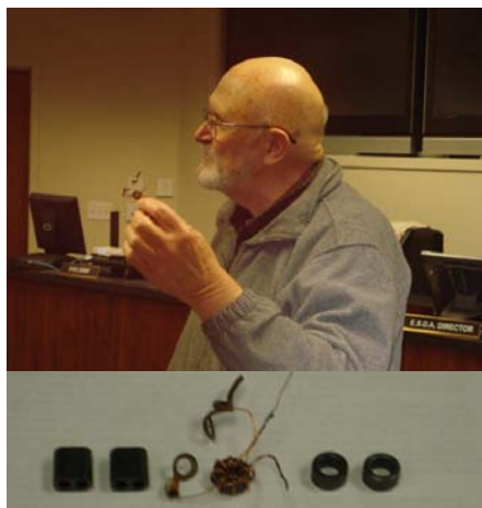
Will K9FO showed how to build receive antenna transformers and the difference and use of Different types of ferrite cores
