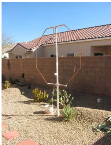
WB9RUE's magnetic wave antenna in the Arizona desert
